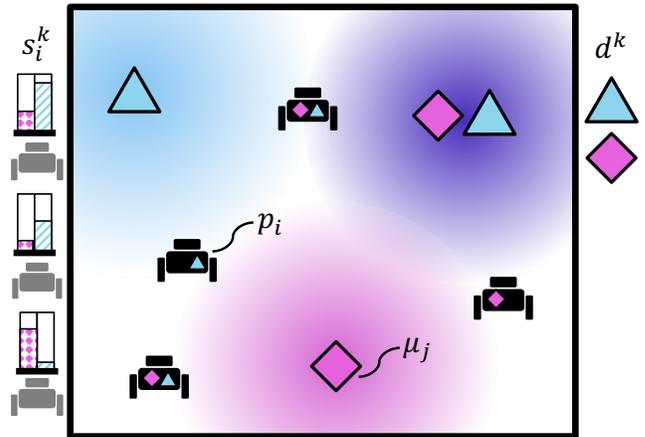
Fig. 2. Our goal is to assign robots with varying supplies to meet varying demand across the environment. In this example, we have three demand locations  $\mu_j$ , each requiring one or both of the resources denoted by the  $\triangle$  and  $\diamond$ . Each robot at location  $p_i$  carries different amounts of resources, and some robots may specialize in one resource type.
