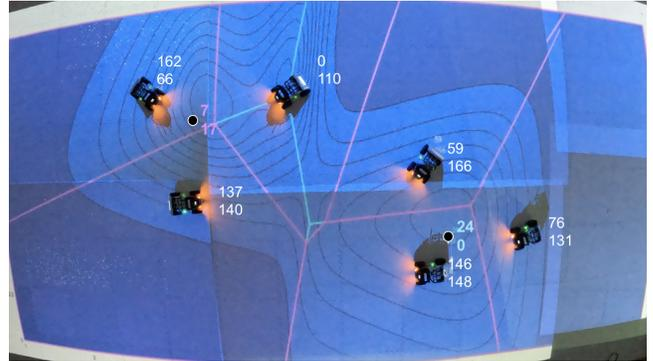
Fig. 1. Our experiments demonstrate a team of 6 robots supplying 2 different types of resources to 2 dynamic locations (o). Quantities of each resource carried/demanded are printed to the right of the robot/o. The contours indicate density in the space, and solid lines represent Voronoi boundaries.
