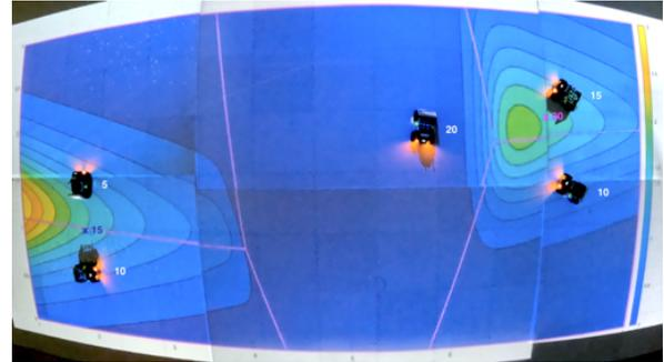
Fig. 1. Final configuration of a team of 5 robots supplying multiple resources of a single type to 2 different locations ( $\times$ ). Quantities of resources carried/demanded are printed to the right of the robot/ $\times$ . The colorbar indicates density in the space on a scale of 0 to 3, and lines represent Voronoi boundaries.
