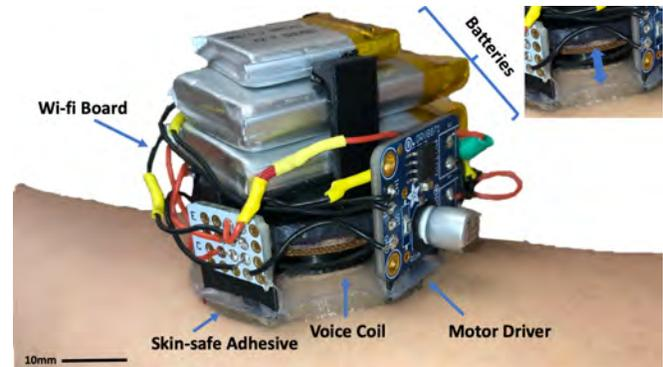
Fig. 8. Probing module with voice coil in a neutral position. The top right image shows a closer view of the voice coil, and the arrow indicates its direction of motion, which is normal to the surface of the skin. The module dimensions are 41mm  $\times$  41mm  $\times$  36mm, and weight is 87g.
