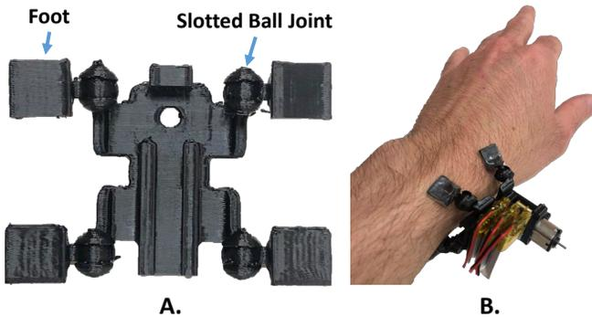
Fig. 2. (A) Slotted ball joints with feet can enable the modules to attach to almost any body location. (B) A module is attached to a user's wrist. The feet are adjusted to match the curvature of the user's wrist.
