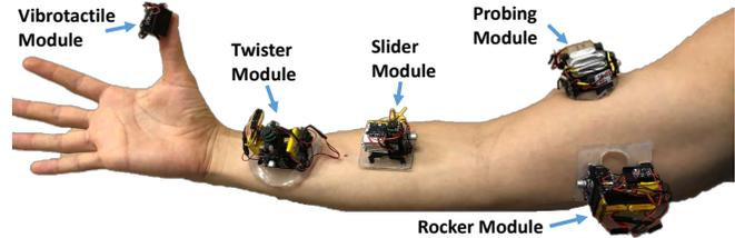
Fig. 1. A user's arm with five self-contained re-attachable haptic modules.
