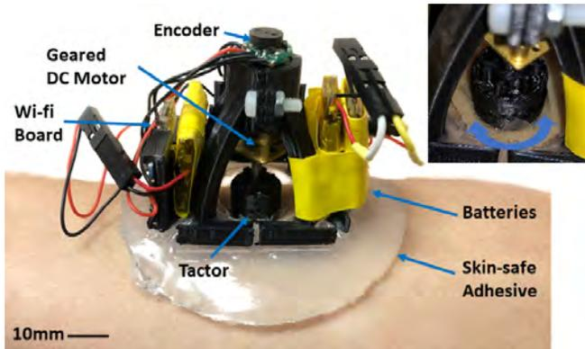
Fig. 6. Twister haptic module. The image in the top right shows a close-up view of the tactor with an arrow indicating that skin-stretch can be generated either clockwise or counterclockwise. The module dimensions are 48mm  $\times$  43mm  $\times$  47mm, and weight is 61g.
