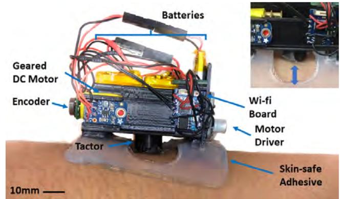
Fig. 4. Rocker haptic module. The tactor's axis of rotation is parallel to the skin's surface and the skin stretches as the tactor rotates about this axis. The module dimensions are 53mm × 27mm × 32mm, and weight is 54g.
