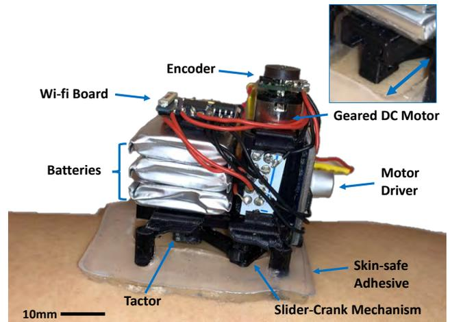
Fig. 7. Slider haptic module. The top-right figure shows a close-up picture of the tactor, and the tactor movement. The module dimensions are 41mm  $\times$  31mm  $\times$  36mm, and weight is 44g.
