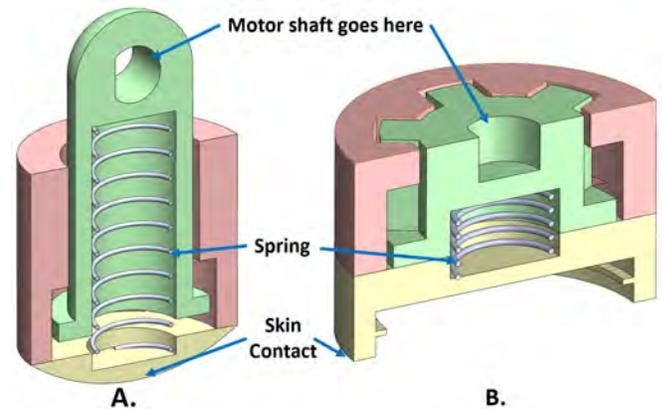
Fig. 5. Cross sections of the spring-loaded tactors for (A) the rocker module and (B) the twister module.
