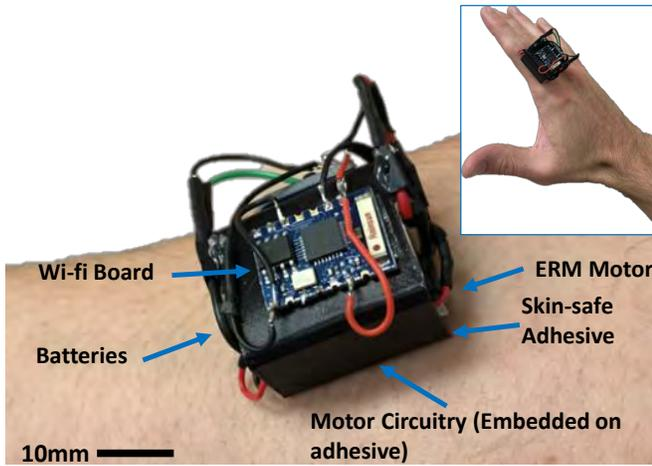
Fig. 3. Vibrotactile haptic module. The top-right figure shows the vibrotactile module on the user's finger for scale. The module dimensions are 25mm × 23mm × 15mm, and weight is 17g.
